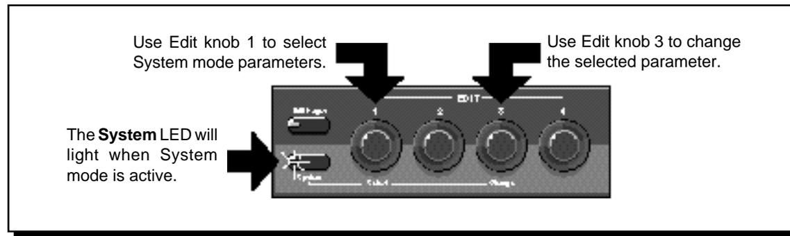
Except for MIDI dumps and reinitialization commands, which require confirmation to execute, system parameter changes are effected immediately.
