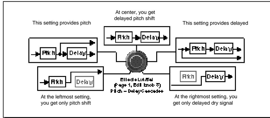
Behavior of **Effects Lvl/Bal** in the cascade programs. Several points from the knob's continuous range are illustrated here, using Pitch-Delay as an example.
