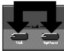
2. Press the front panel button you want to control (**Bypass** or **Tap**).
