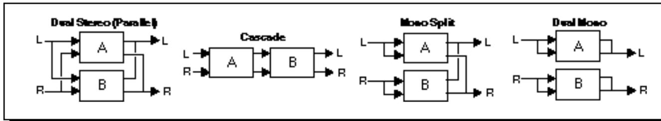
Generally, the **Effects Lvl/Bal** parameter (Page 1, Edit knob 3) controls the balance of the two effects in each dual program. In the cascade variations, rather than simply controlling balance, the knob varies the amount of the first effect or dry signal which is fed into the second effect.
