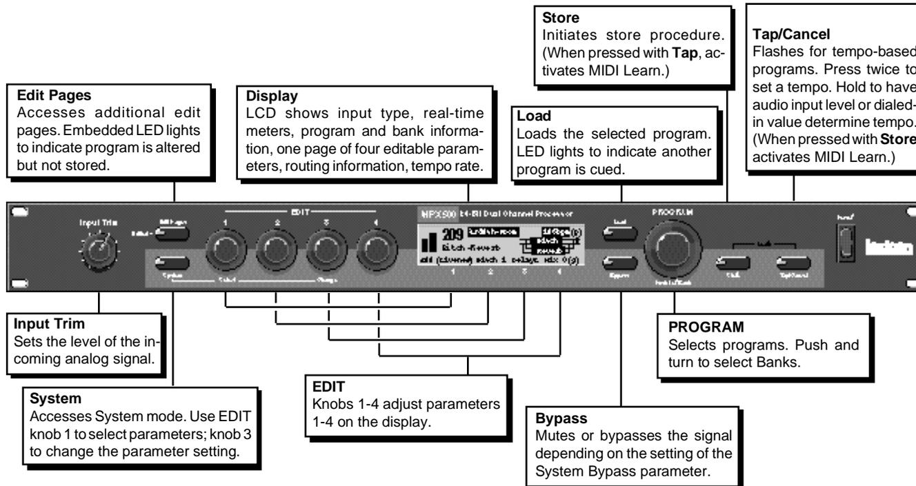
\* The level indicators are at their minimum size when the incoming signal is low (more than 30dB below full scale). The highest level indicators are highlighted when the signal approaches full scale.
